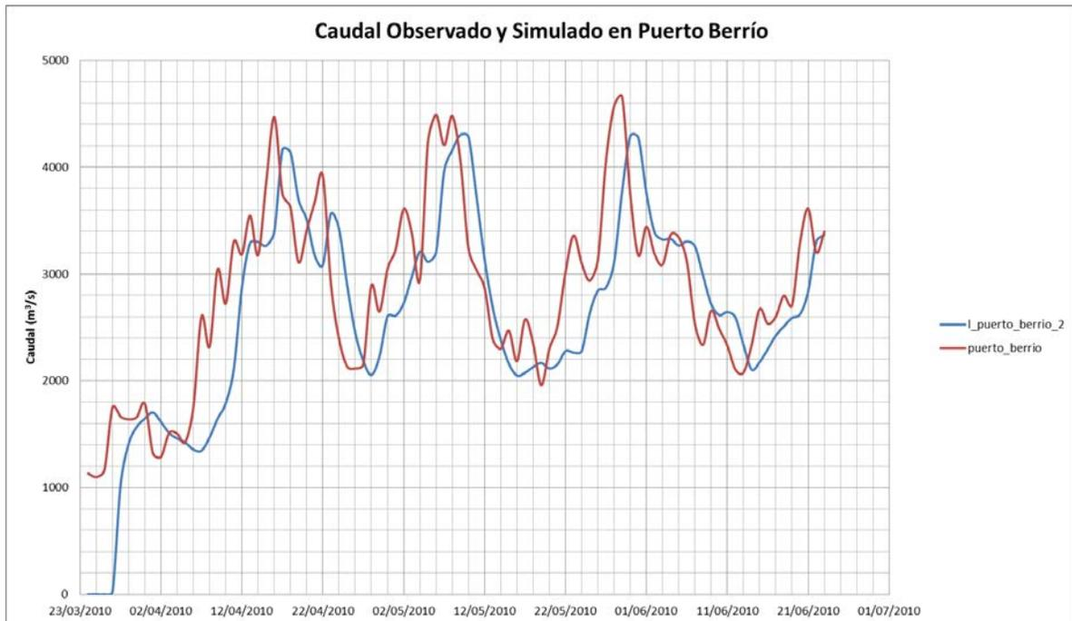
Fig. 13 Measured Flow in Puerto Berrio station 23097030 (Red) and simulated for Puerto Berrio section 2D Flow Model
