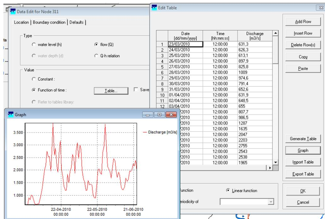
Fig. 5 Condition Border sub model 1 Upstream. Puerto Salgar flow Station 23037010.
