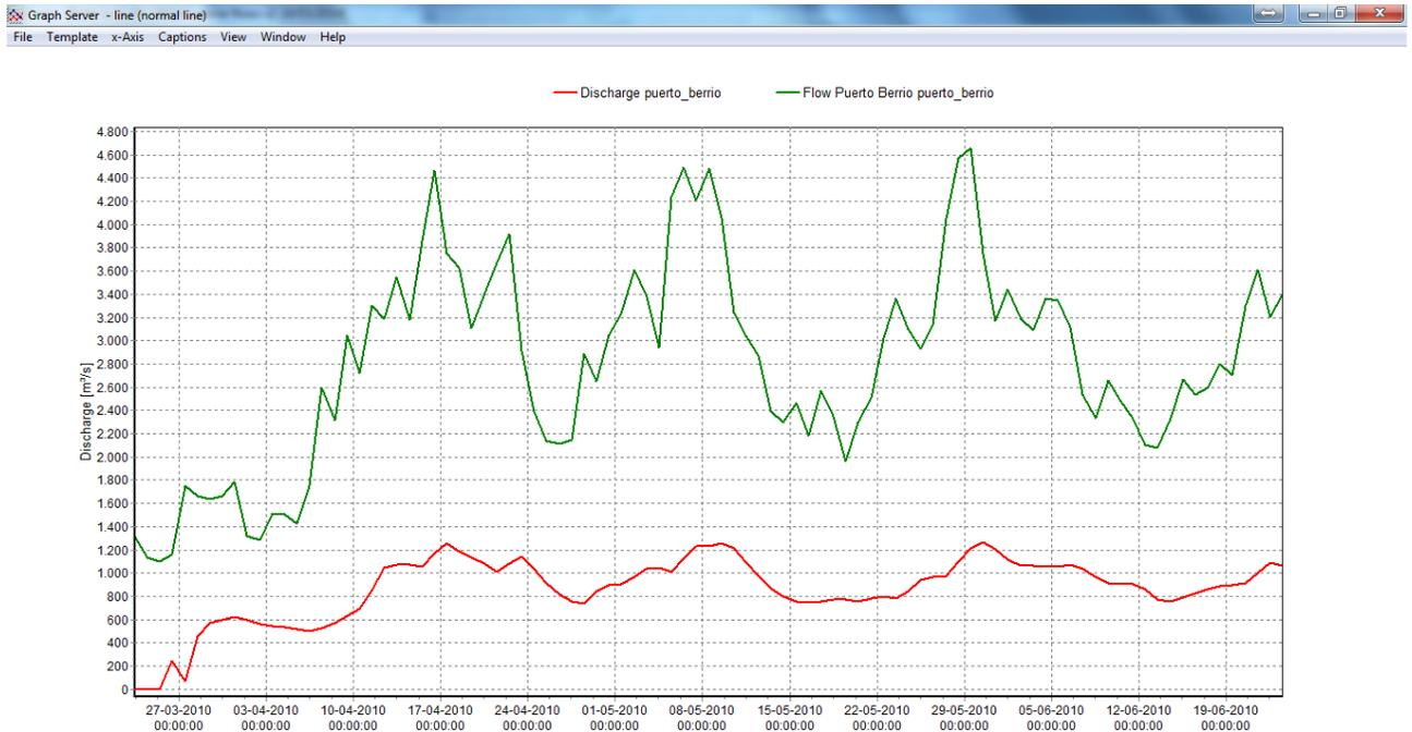
Fig. 12 Measured flow at station 23097030 Puerto Berrio (Green) and simulated for Puerto Berrio section 1D Flow Model.
